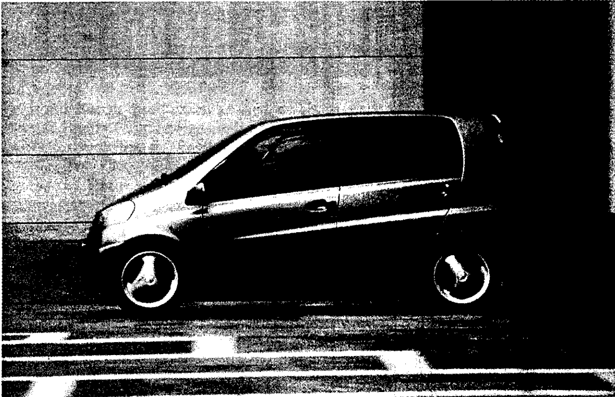
FIGURE 9.14. Mercedes-Benz zero emission class A EV. The car uses a 40 kW (54 hp)—three phase induction motor developing a rated torque of 155 Nm which can accelerate the car to 100 km/h in 17 sec with a top speed of 120 km/h and a normal usage range of 150 km. Recharging can be made in 6–12 h using normal household sockets. The battery system is sodium/nickel chloride with an energy storage capacity of 100 Wh/kg and a life of over 100,000 km.
