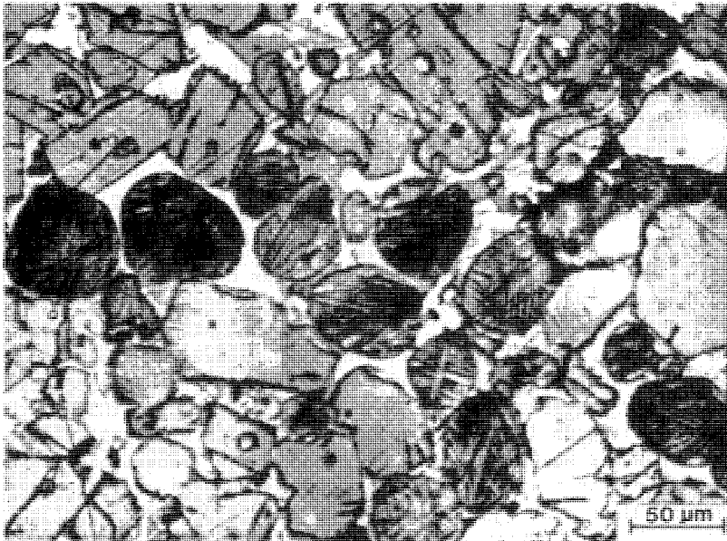
Fig. 4.2 Reflected light micrograph of a polished and etched section of a Portland cement clinker, showing crystals of alite (angular) and belite (rounded and striated) embedded in a matrix of interstitial material, itself composed mainly of ferrite (light) and aluminate (dark). Courtesy Materials Science Department, British Cement Association.
